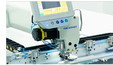
电子随动压脚防止跳线和断线 Electronic follower foot prevents thread skipping and thread breakage
